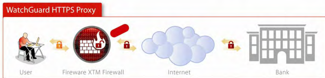
Figure 2: When a user behind a WatchGuard Fireware XTM firewall makes the same request as in Figure 1 to receive encrypted data, the firewall is able to decrypt the HTTPS traffic into normal HTTP. It can then inspect it for anomalies, re-encrypt the data, and pass it along to the user. The user’s communication remains confidential, while the network has an additional layer of protection from encrypted threats.
